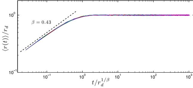
**Fig. 2.** Surface roughness rescaled by the target value  $r_d$  against the rescaled time  $t/r_d^{1/\beta}$  for all cases shown in Fig. 1. The dashed line corresponds to a guide-to-eye line with slope 0.43.
