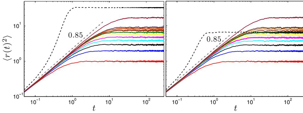
**Fig. 1.** Squared value of the surface roughness of the solutions to the sKS equation with Burgers nonlinearity (left) and the KPZ nonlinearity (right) for  $\nu = 0.05$ ,  $\sigma = 0.5$  and different values of the desired surface roughness, ranging from 1 to 10, and 20. The dashed lines show the value of the uncontrolled roughness, and the straight dashed-line corresponds to a guide-to-eye line with slope 0.85.
