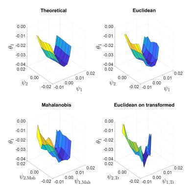
FIGURE 6. Estimation of the first drift coefficient  $\theta_1$ . "Theoretical" are obtained numerically from (5), "Euclidean" via DMaps on the original data, and "Mahalanobis" from DMaps on the transformed data. The last subplot shows results from Euclidean DMaps on transformed data, which, as expected, yields incorrect estimates.
