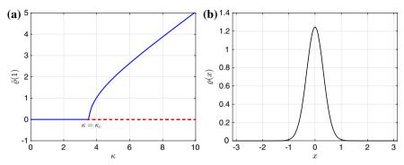
**Fig. 2.** a The bifurcation diagram for the noisy Kuramoto system: the solid blue line denotes the stable branch of solutions while the dotted red line denotes the unstable branch of solutions. **b** An example of a clustered solution representing phase synchronisation of the oscillators
