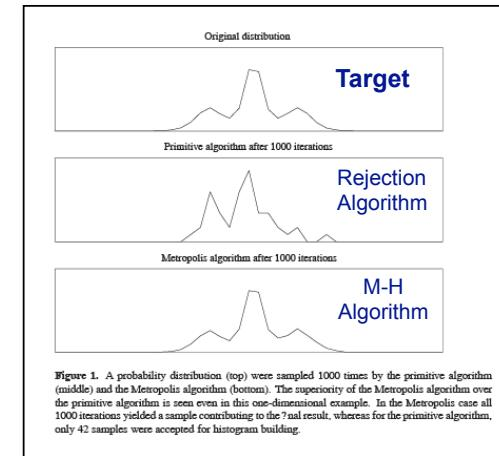
Figure 1. A probability distribution (top) were sampled 1000 times by the primitive algorithm (middle) and the Metropolis algorithm (bottom). The superiority of the Metropolis algorithm over the primitive algorithm is seen even in this one-dimensional example. In the Metropolis case all 1000 iterations yielded a sample converging to the ?nal result, whereas for the primitive algorithm, only 42 samples were accepted for histogram building.
