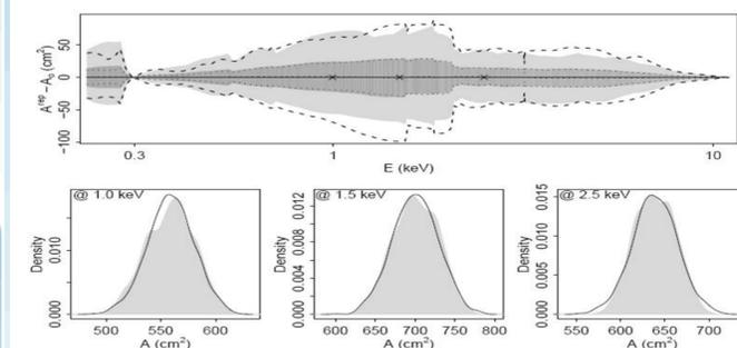
**FIGURE 2:** The grey regions in the upper panel give intervals for each energy bin that contain 100% and 68.3% of the calibration sample. The dashed and dotted lines outline intervals for each energy bin containing 100% and 68.3% of 1000 PCA replicates of the effective area. The bottom panel details the comparisons between the calibration sample and PCA summary for the particular energy bins.
