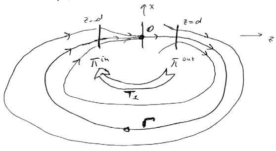
Note that the flight time from  $\Pi^{in}$  to  $\Pi^{out}$  tends to infinity as  $\varepsilon \to +0$  (would it remain finite, we would take a limit and obtain orbits which come from  $\Pi^{in}$  to  $\Pi^{out}$  at  $\varepsilon = 0$ , but such do not exist). This implies that the map  $T_0$  is a strong contraction. Indeed, at  $\varepsilon = 0$  at the point O the linear part of the system is
