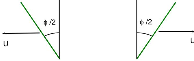
Figure 7.17: Schematic diagram for the spreading out phase of the Weis-Fogh mechanism. Both wings are separated by an angle  $\phi(t)$  at their lowest point and move away from each other with relative speed  $2U$ .
