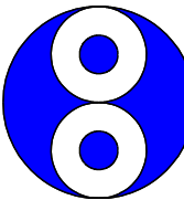
Fig. 5.7: A continuous branch of rotating vortex arrays connecting the co-rotating point-vortex pair to the Rankine vortex. The sixth figure is the limiting state of the solution where \rho = \rho_{crit} and where the two patches develop cusps and touch at 3 distinct points enclosing circular irrotational regions centred on the point vortices. The last two figures illustrate the desingularization of the point vortices to form a single Rankine vortex. The circulations \Gamma_s and \Gamma_{sp} of respectively the satellite point vortices and vortex patches are also shown.
