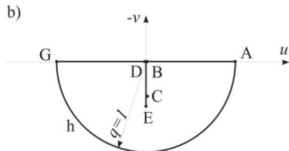
Open hollow wake without corner separation: a) physical plane; b) hodograph plane.
