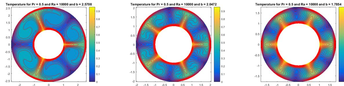
We can clearly see the cells of convection that have been formed. As the annulus size decreases we get more rolls of convection, this is because as  $b \rightarrow 1$  we approach Rayleigh-Bénard convection in an infinite layer.
