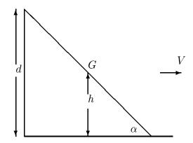
A tube train travels with speed V > 0 along the x-axis. A passenger is leaning backwards against a smooth wall at an angle  $\alpha$  as in the diagram, when the train begins to decelerate at a constant rate. The man's centre of mass G is a height h above the floor, while his back touches the wall at a height d > h. The coefficient of friction between his feet and the floor is  $\mu$ .
